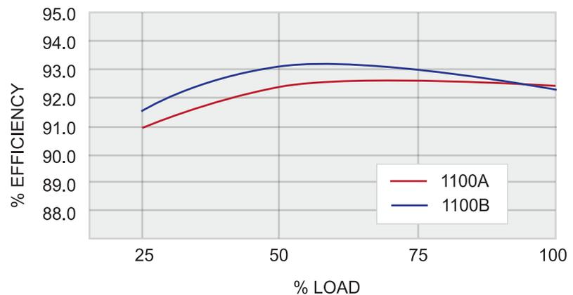
*The efficiency of the compact DiamondPlus™ 1100 Series peaks at over 93% at a nominal operating range.*
